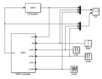
If any of these inports are unconnected, their associated variables are treated as unbounded signals. The corresponding variable in the mpc object must also be unbounded.
