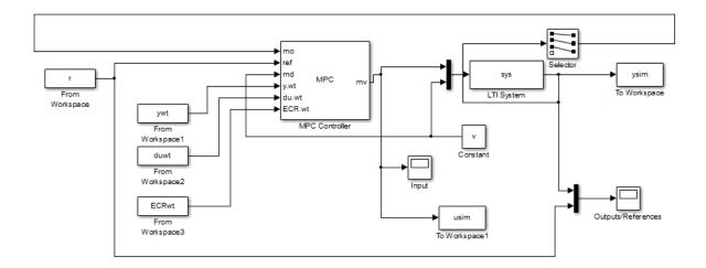
Add an inport (y.wt) for a vector signal with  $n_y$  elements. Each element specifies a nonnegative tuning weight for each controlled output variable (OV). This signal overrides the MPCobj. Weights.OV property of the mpc object, which establishes the relative importance of OV reference tracking.
